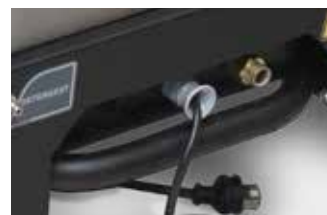
Front and rear protective bumper also useful for improving maneuverability and safety in manual lifting operations
